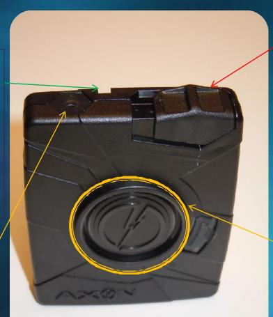
On/Off Slider Red = On/Buffering Pre-Event Buffering/Pre-Record is for 30 seconds prior to double tapping record button – Video only during 30 second buffer then audio and video.
